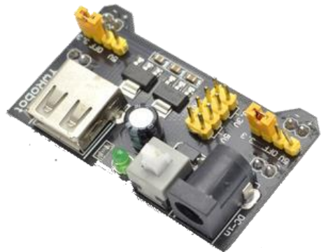
Fig 4.2.3c: HW-131 POWER SUPPLY
